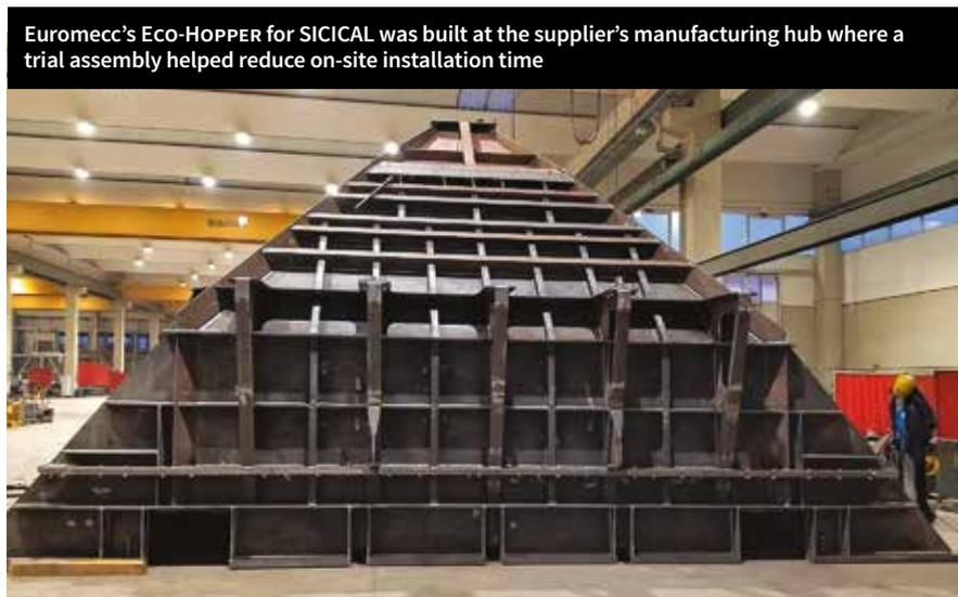
Euomecc's ECO-HOPPER for SICICAL was built at the supplier's manufacturing hub where a trial assembly helped reduce on-site installation time
