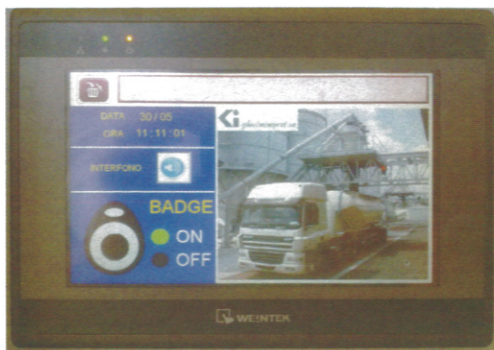
Touchscreen for the unloading inside the rail wagon.
