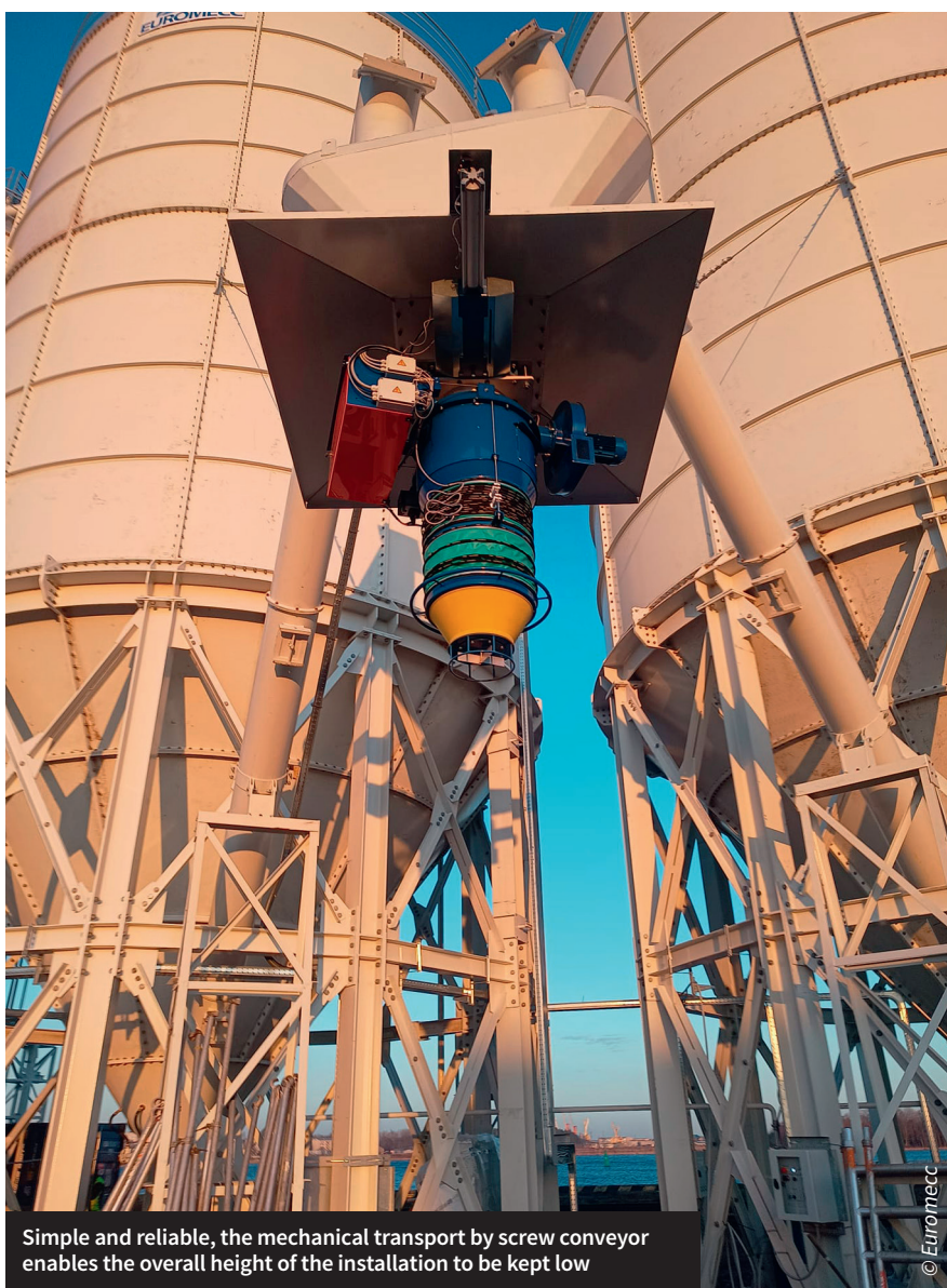
Euromecc's design minimises the number of horizontal connections so that there is only one intermediate flange, making everything safer and simpler
